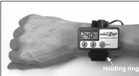
Fig. 4: Fix miniZAP ® on the wristband and plug the cable into the output socket.
